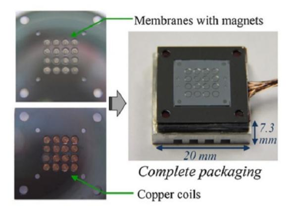
*Figure 1 -* 4×4 micro-actuator array: mounting and integration into its packaging [2].
