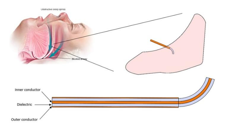
Figure 2 - Soft Palate model with the open-tip antenna
