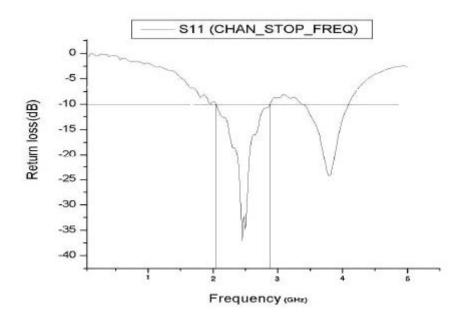
Figure 5 - Variations of the measured reflection coefficient at the antenna's port
