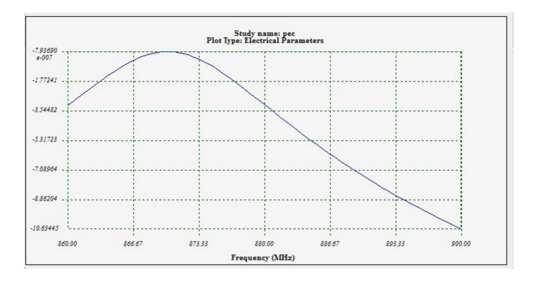
Figure 3 - Insertion (Bottom) and return (Top) losses
