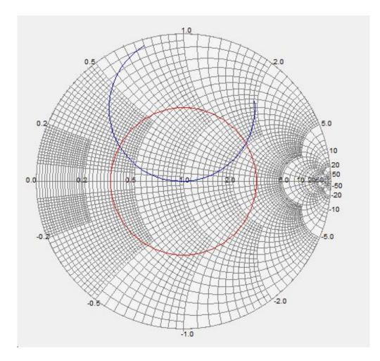
Figure 4 - S11 plot on a Smith Chart (880 MHz)
