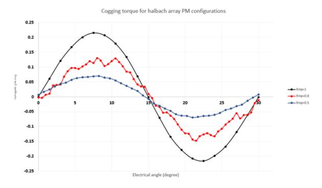
Figure 4- Cogging torques versus electrical angle
