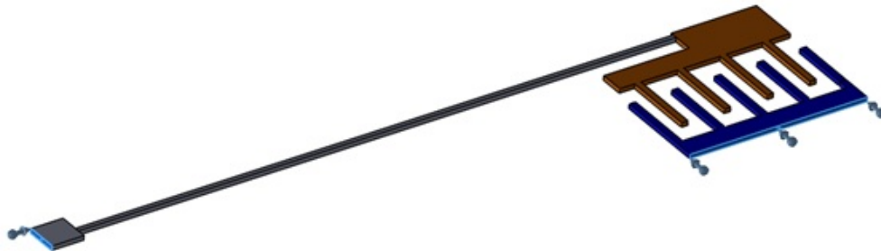
Figure 4 - Fixed constraint applied on the fingers
