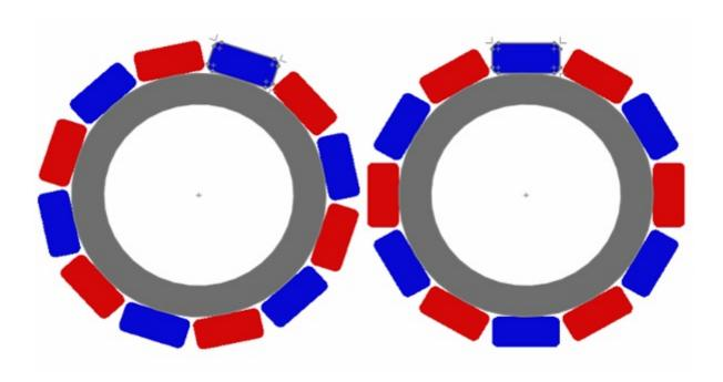
Figure 7 - Magnetic gear model with parallelepiped poles
