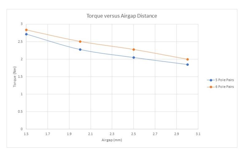
Figure 12 - Torque results versus airgap distance
