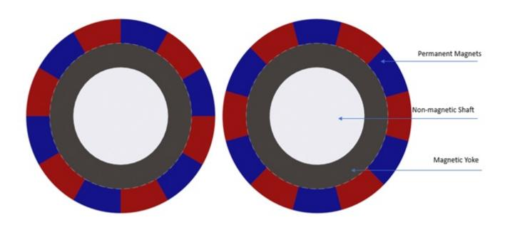
Figure 1 - Magnetic gear model with radial magnets
