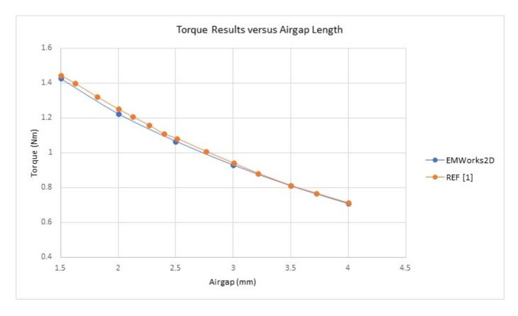
Figure 6 - Torque results versus airgap distance
