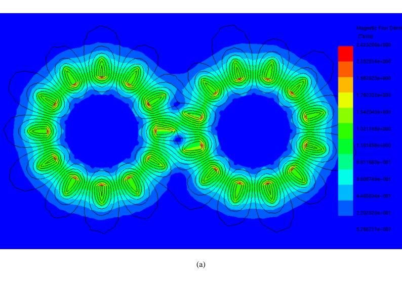
Figure 2 - Magnetic flux density at different positions, a) 0 deg, b) 15 deg, c) 45 deg
