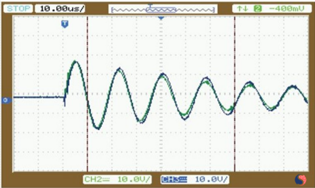
Fig. 4. Current Waveform at 9KJ Discharge Energy [2]
