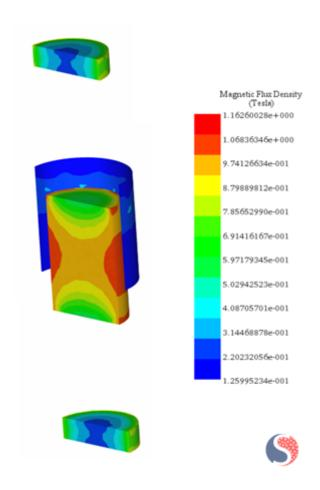
Fig. 12. Magnetic Flux Density Distribution - Topology 1
