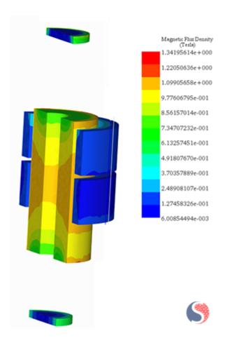
Fig. 14. Magnetic Flux Density Distribution - Topology 3: Uniform Magnetization
