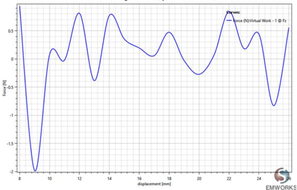
Fig. 9. Restoring Force - Topology 3: Halbach Magnetization
