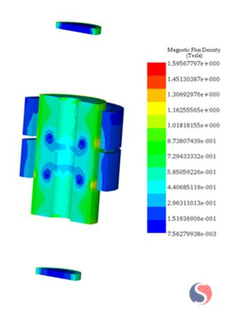
Fig. 15. Magnetic Flux Density Distribution - Topology 3: Halbach Magnetization
