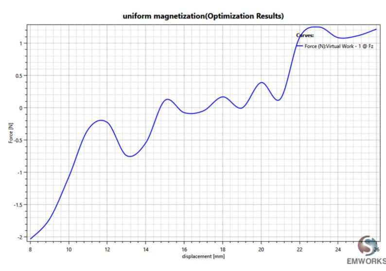
Fig. 8. Restoring Force - Topology 3: Uniform Magnetization
