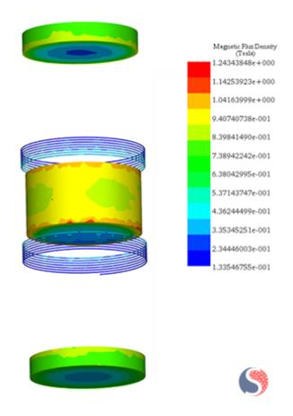
Fig. 13. Magnetic Flux Density Distribution - Topology 2  $\,$
