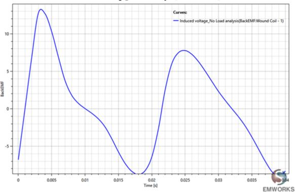
Fig. 10. Induced Voltage in a Single Coil
