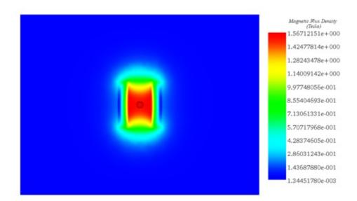
Figure 10 - Magnetic flux density created by a bore coil
