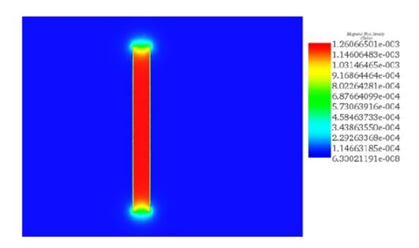
Figure 4 - Magnetic flux in reference coil
