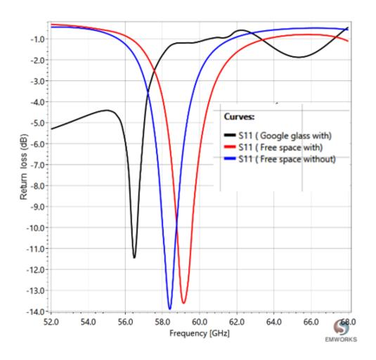
Fig.6. Return Loss of the Antenna
