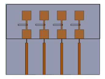
Fig. 1. Geometry of the mmWave Patch Antenna Array with Parasitic Elements
