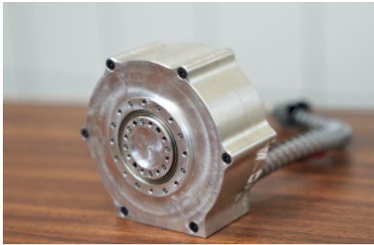
Fig. 1: BEAR: Back-drivable Electromechanical Actuator for Robotics
